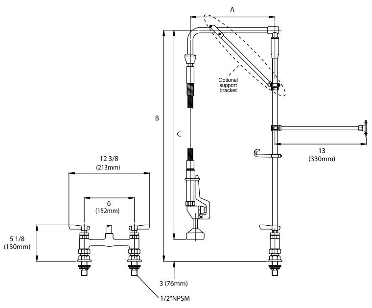
1-1/8" (29mm) holes for deck are recommended to accommodate 1/2" supply nipples.
